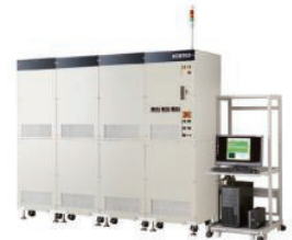
Charge/discharge testing system (2019)
